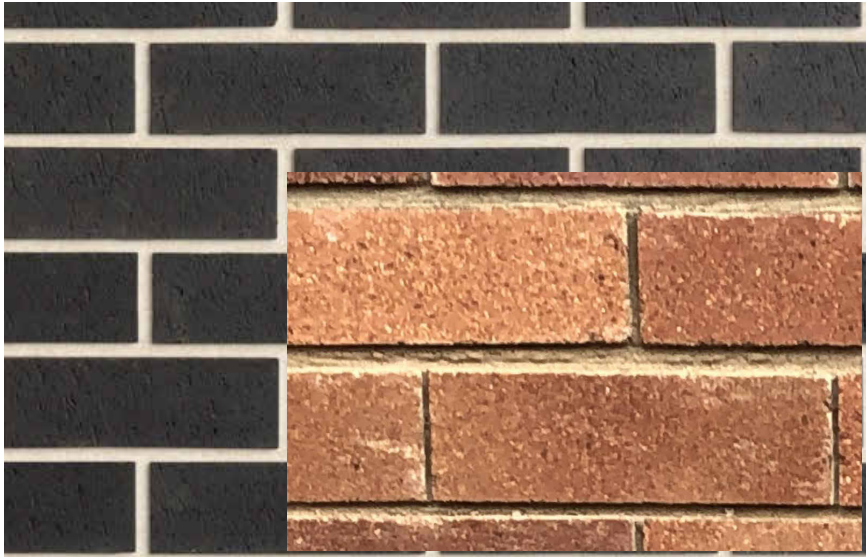
BWK BUILDING BASE CLADDING - FACE BRICKWORK + 2% RECYCLED BRICKS FROM SITE
